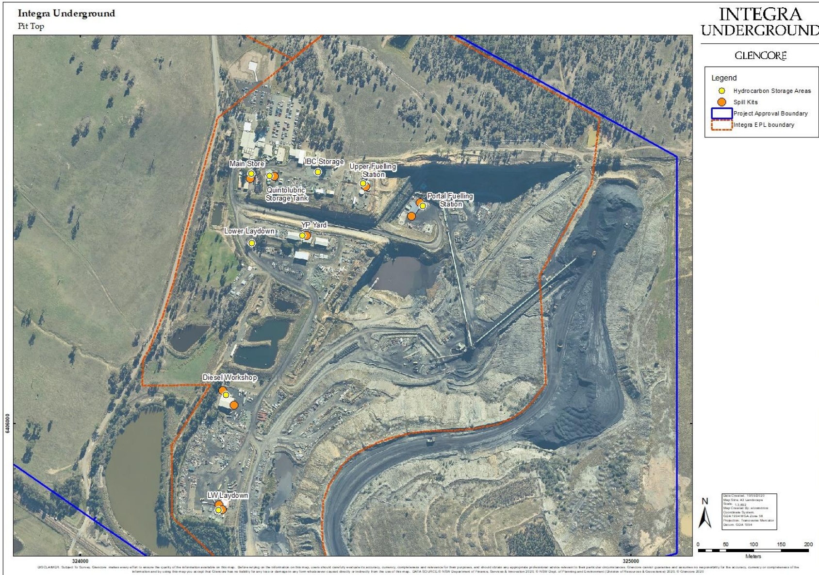
Figure 5 – Spill Kit and Hydrocarbon Temporary/Fixed Storage Locations
