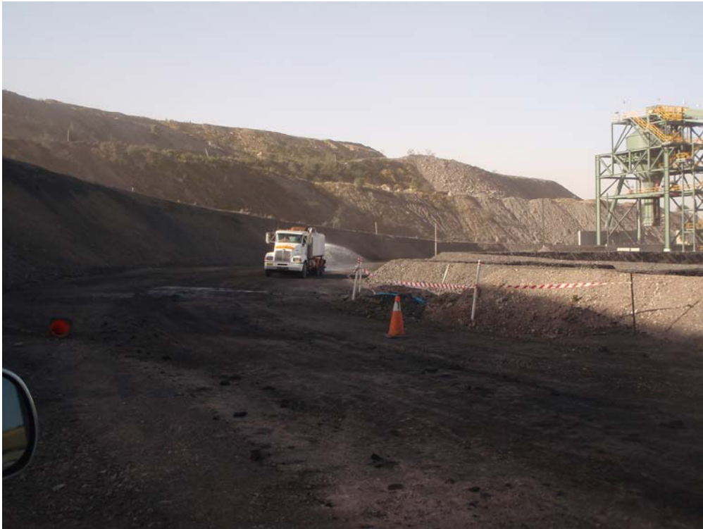
Plate 5 Active dust suppression - watercart on the haul road
