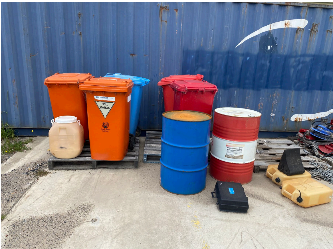
Photo 8 – Old drums behind dollar shed should be stored within a bund.
