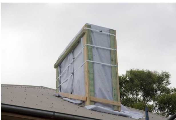
Figure 12 Main chimney frame (plus framing below roof) Accelerometer locations
