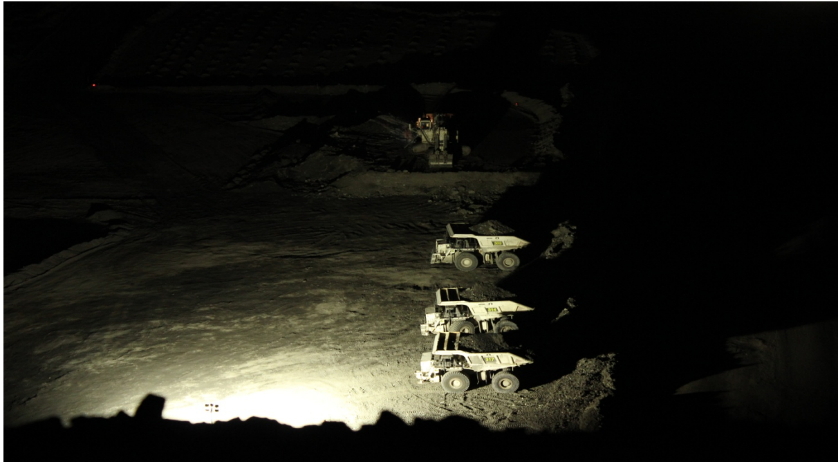
Photograph 3.3 Temporary lighting plant used to illuminate work area in the pit and overburden dumps
