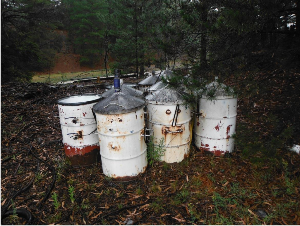
Photo 15 – Chemical Containers stored outside a bund adjacent to a laydown area
