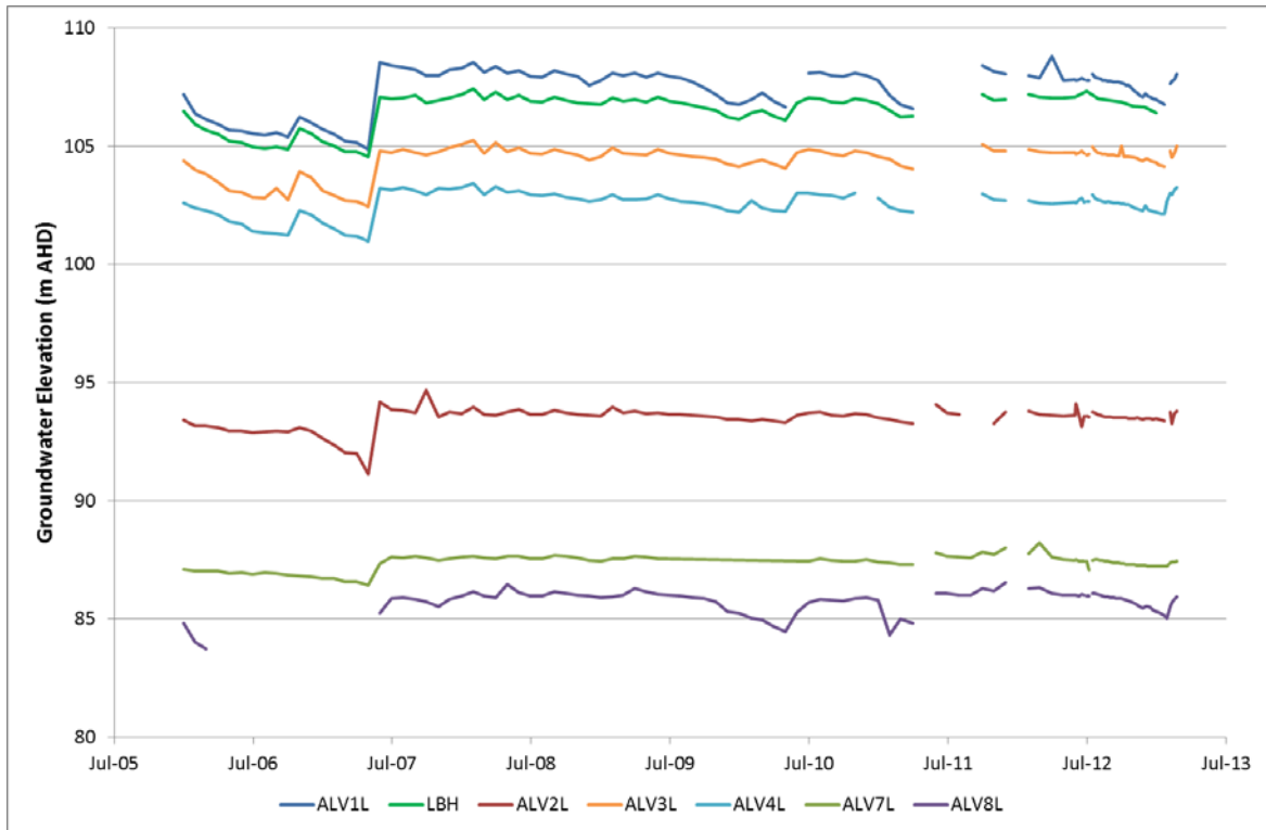
Figure 38 Groundwater Levels for Alluvial Piezometers – 2006 to 2012
